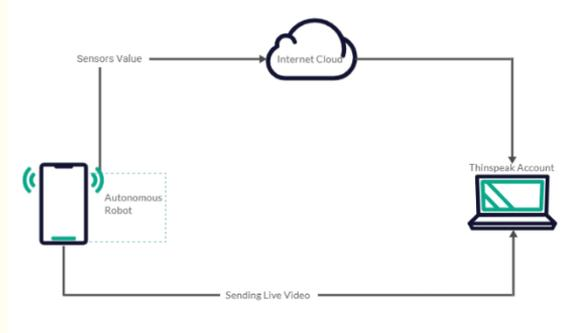
Figure 1. Block Diagram for Communication with Surveillance and Rescue Robot
