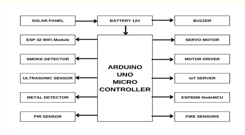
Figure 2. Block Diagram for IoT Based Surveillance and Rescue Robot
