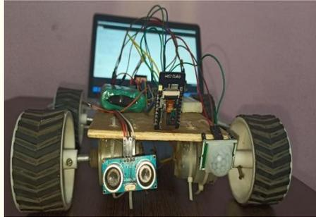
Figure7. Prototype of IoT Based Surveillance and Rescue Robot with sensors
