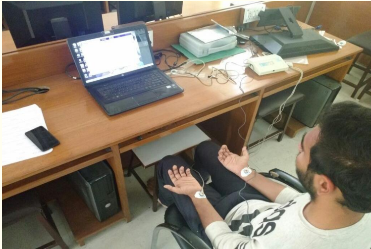
Figure 3.ECE and Respiration signal acquiring set up
